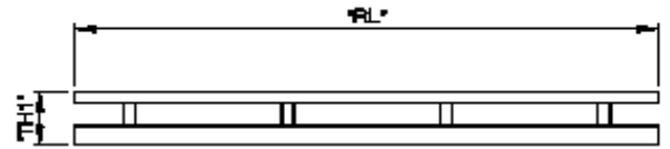
Truss Track Runway
